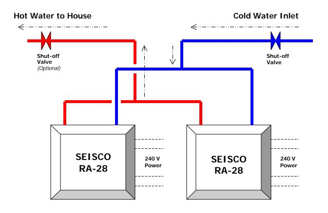
Both Seisco Tankless Water Heaters for this configuration should be the same Model or size. At 240 Volts, two RA-18's = 36 KW, two RA-22's = 44 KW and two RA-28's = 56 KW maximum power output.
