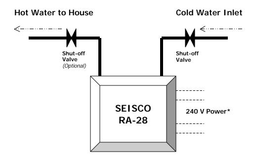
\* The RA-28 Model requires **FOUR** 30 Amp, 240 Volt circuits from the main electrical panel or from an installed sub-panel or disconnect box.
